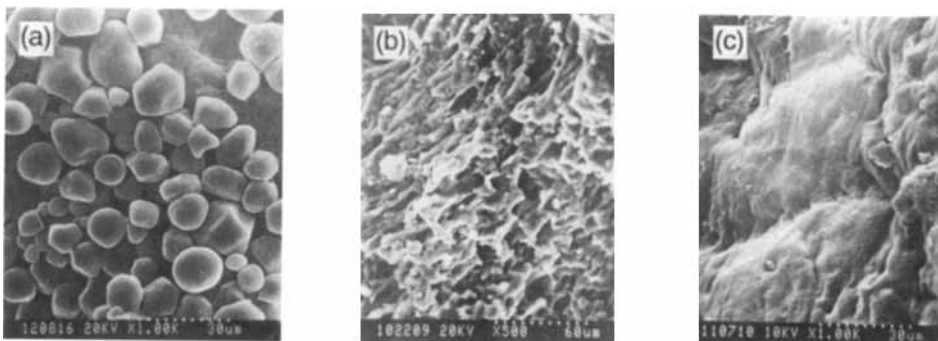
Figure 7. SEM of starch (a), starch-g-PAA (b), starch-g-AM (c), starch-g-PMMA (d), starch-g-PAN (e).
